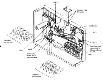
REMOVE THE APPROPRIATE CABLE ENTRY CUT-OUTS BEFORE FIXING THE BOX, WHERE POSSIBLE DRILL THE BOX TO PROVIDE A CLOSE FITTING ENTRY FOR CABLES AND HEAT-RESISTANT FLEXIBLE CORDS. TAKE CARE TO REMOVE SHARP EDGES.
